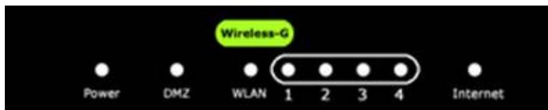
Be patient; the DMZ indicator will eventually go out. When it does, your router has been converted! The router will take about two full minutes to re-boot from flash, so bide your time during this process.
